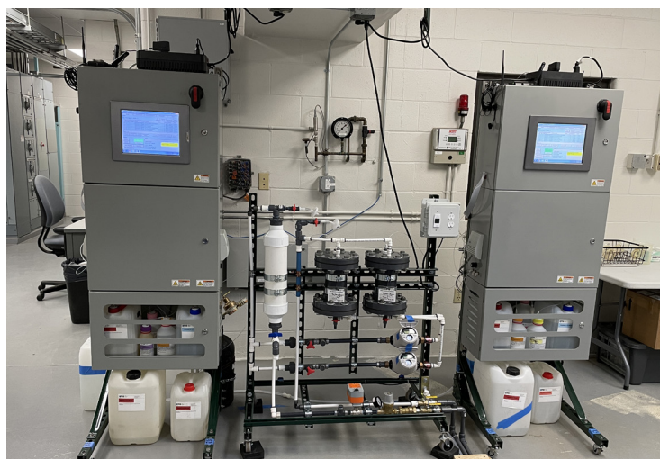
Shown are two MetalGuard™ analyzers operating within the integrated MetalGuard PRS system, one dedicated to lead and one to copper.
